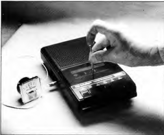
Figure 1: Adjusting the azimuth setting using a small screwdriver and milliammeter
